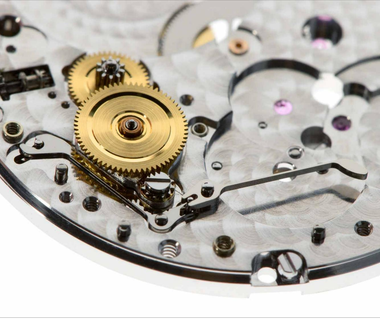
In the foreground the full hacking system for the balance wheel, starting on the left from the setting lever. Behind it, the first, star-shaped toothed pinion (known as a Pelton gear) meshes with the lower level of the gold coloured reverser wheel. Allowing this level to turn in only one direction. The pinion behind it then meshes with the pinion set into the barrel bridge which inturn winds the ratchet wheel and mainspring. The rotor winds the watch as it rotates in both directions.
